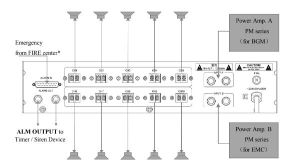
\*ALARM IN to be connected to fire center
